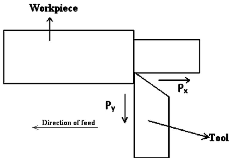
Figure 4: - top view of cutting action
