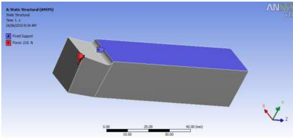
**Figure 8:- fixed support given to the tool.**
