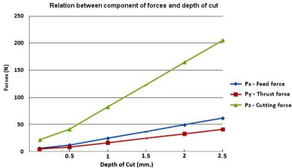
**Figure 5:-graph of components of cutting forces vs. depth of cut**
