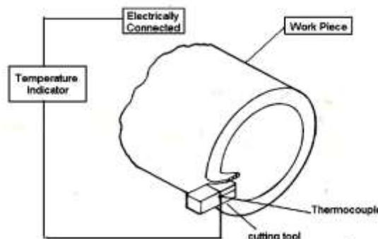
**Figure 1:-Temperature Measurement in Metal Cutting**
