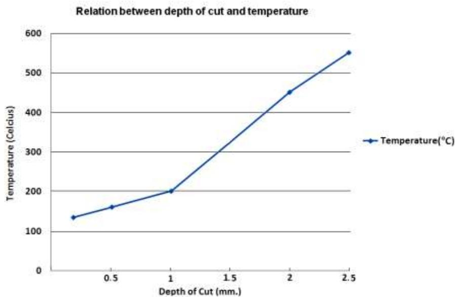
**Figure 2: - graph of temperature vs. depth of cut**
