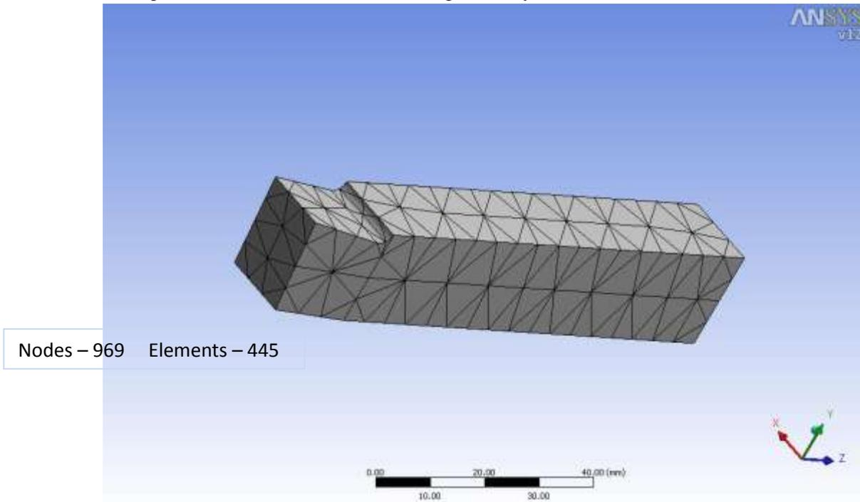
Figure 7:- mesh model made by ansys software
