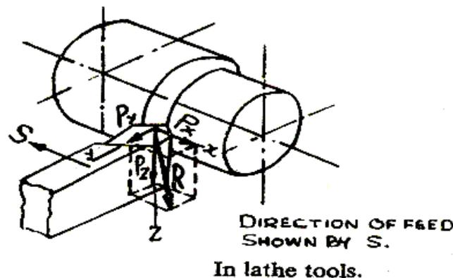
**Figure 3: - components of cutting forces**
