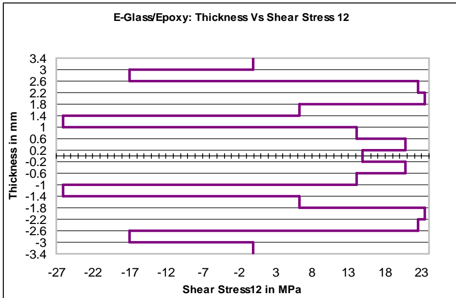
Figure 9.12 Variation of \tau_{12} through thickness of E-Glass/Epoxy Drive Shaft
