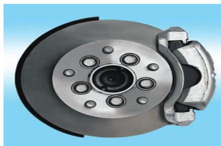
Fig.1 ventilated disc brake and assembly
