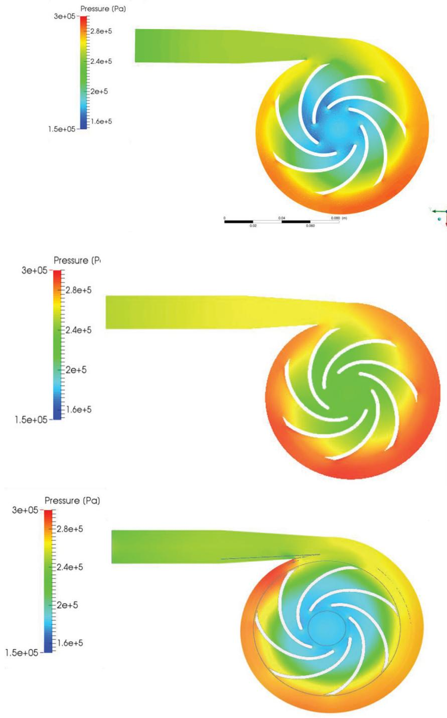
Figure 2 Mid-height pressure contour in case of tomato paste processing
