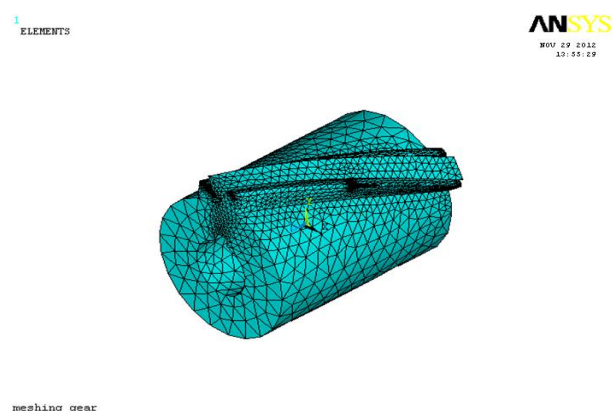
Fig 3 Meshing of Contact gear model
