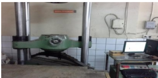
Figure 7: Experimental Setup of Leaf spring on the UTM
