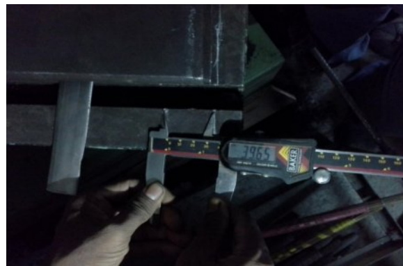
Figure 8: Deflection in the leaf spring
