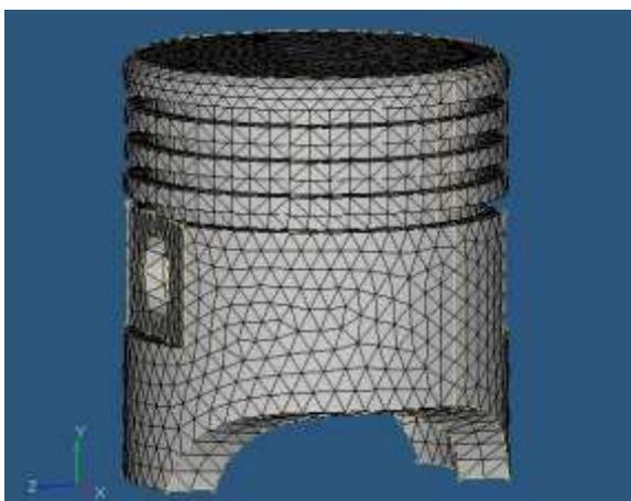
Figure 7. Meshing on Piston
