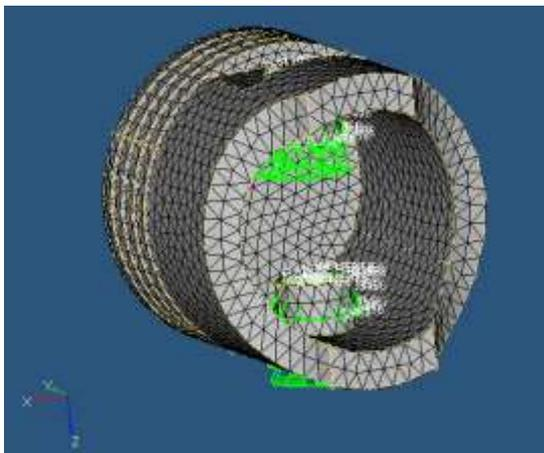
Figure 6. Boundary Conditions on Piston
