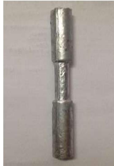
*Figure 2.specimen of Al-Sic-Graphite*
