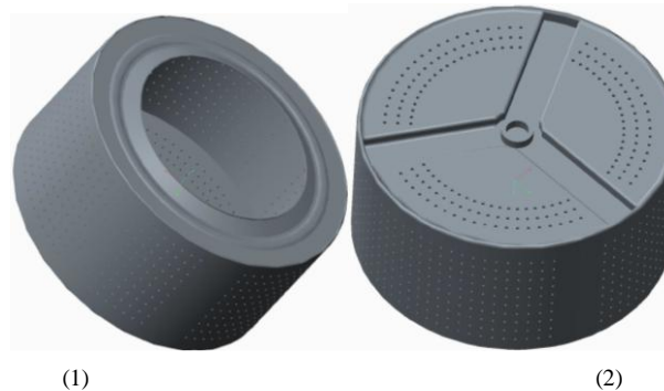
Fig. 1. Different views of the Washing Machine Drum
