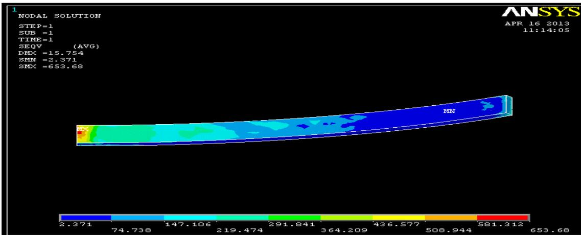
Fig.4- Von-mises stresses of Graphite leaf spring
