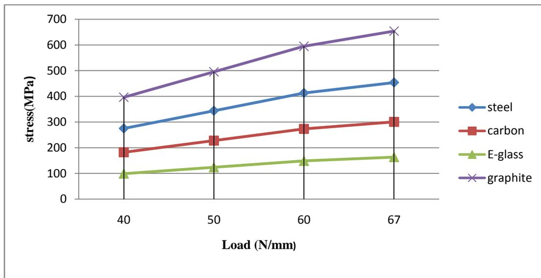
Fig.6: Stress Vs Load
