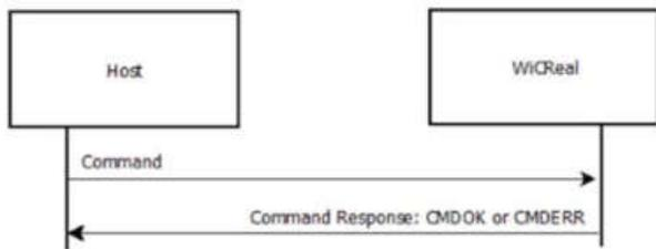
Figure 5. Command does not generate an event.
