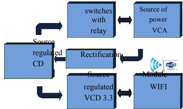
Figure 11. Block diagram of Smart Switch.
