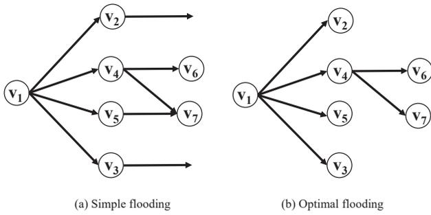
Fig. 4. The formalization of flooding problem.
