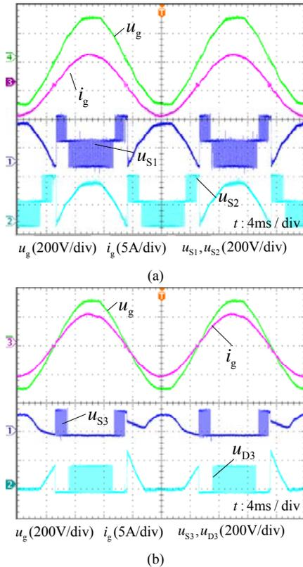
Fig. 18. Experimental waveforms of the SD five-level DBFBI. (a)  $u_{S1}$  and  $u_{S2}$ . (b)  $u_{S3}$  and  $u_{D3}$ .
