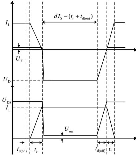
Fig. 12. Hard-switching waveforms of MOSFETs for loss calculation.
