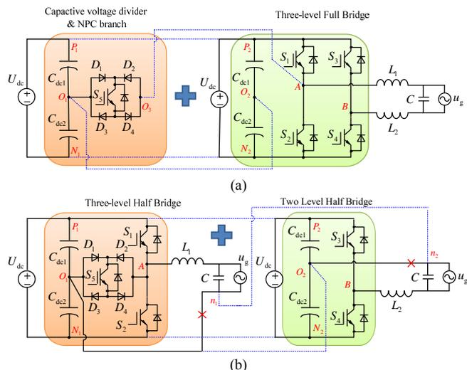
Fig.4. The topology generation rules of the simplified five-level H-bridge inverter. (a) Three-level full-bridge inverter combined with a two-level capacitive voltage divider and a NPC branch. (b) Three-level half-bridge inverter combined with a two-level half-bridge inverter.
