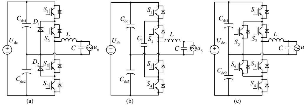
Fig. 1. Three popular topologies of H-bridge multilevel inverters. (a) Diode neutral point clamped (DNPC). (b) Flying capacitor clamped (FCC). (c) Active neutral point clamped (ANPC).
