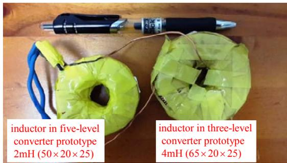
Fig. 16 The filter inductors used in the three-level DBFBI and the five-level DBFBI.
