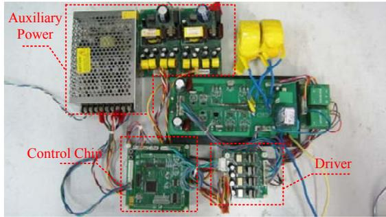
Fig. 15 Picture of the universal prototype.
