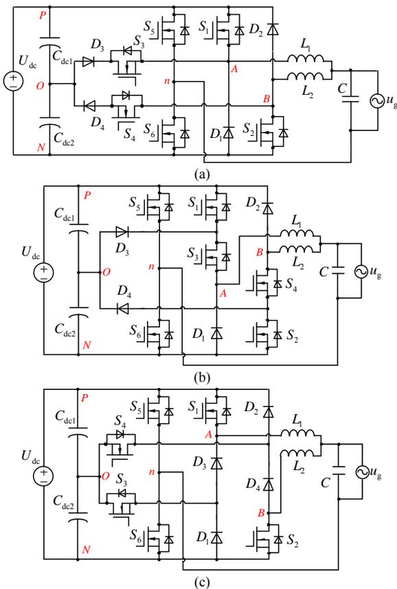
Fig. 3. Three topologies of five-level DBFBIs proposed in [27]. (a) NPC five-level DBFBI. (b) Series-switch five-level DBFBI. (c) Series-diode five-level DBFBI.
