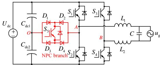
Fig. 2. The simplified five-level H-bridge inverter topology [24]
