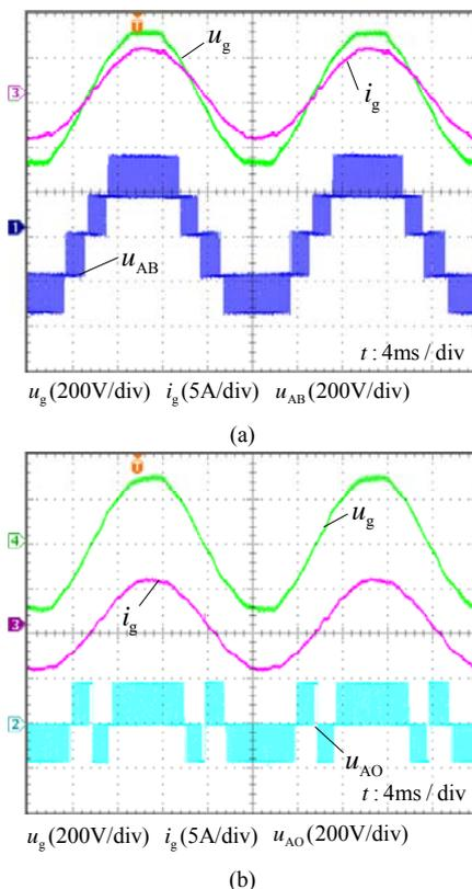
Fig. 19. Experimental waveforms of the conventional five-level H-bridge inverter. (a)  $u_{AB}$ . (b) phase voltage.
