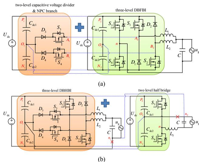
Fig.5. The topology generation rules of the proposed NPC five-level DBFBI topology. (a) A three-level DBFBI combined with a two-level capacitive voltage divider and a NPC branch. (b) A three-level DBHBI combined with a two-level half-bridge inverter.
