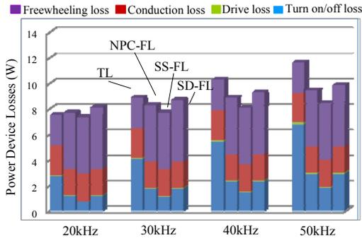
Fig. 13. Total power device loss distributions of four DBFBI topologies under different switching frequencies.
