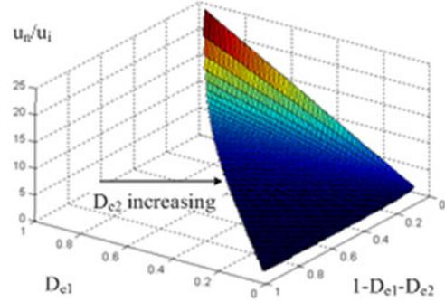
Fig. 5. Relationship between duty ratio of equivalent switch period and voltage step-up ratio.
