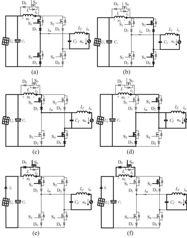
Fig. 4. Equivalent circuit and steady principle waveform of the inverter. (a) Magnetizing state for  $i_m > 0$ . (b) Magnetizing state for  $i_m < 0$ . (c) Regenerating energy state for  $i_m > 0$ . (d) Regenerating energy state for  $i_m < 0$ . (e) Freewheeling state for  $i_m > 0$ . (f) Freewheeling state for  $i_m < 0$ . (g) Steady principle waveform within a LF output period.
