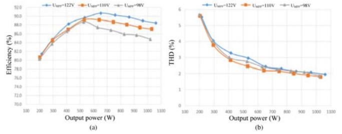
Fig. 8. Conversion efficiency and grid-connected current's THD of the proposed inverter under three kinds of different MPP voltage. (a) Conversion efficiency. (b) Grid-connected current's THD.
