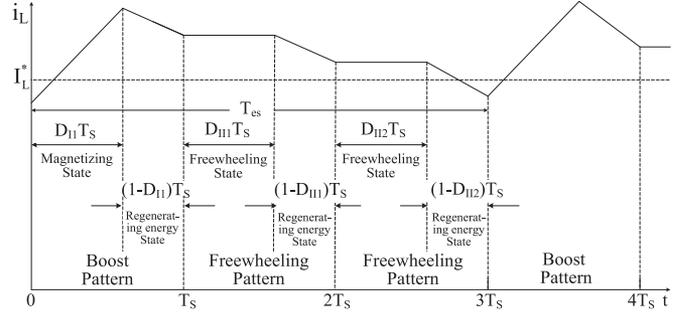
Fig. 2. Waveform of energy storage inductor current with free-wheeling pattern.
