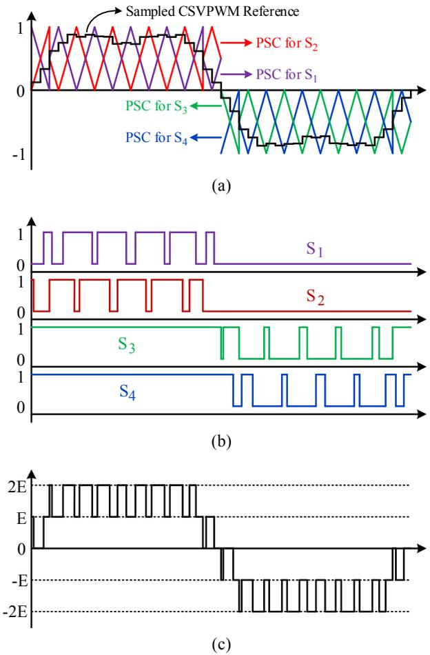
Fig. 3. Carrier-based modulation using modified PSC with sampled CSVPWM reference for three phase application. (a) Reference and carriers arrangement. (b) Gate signals. (c) Output waveform.
