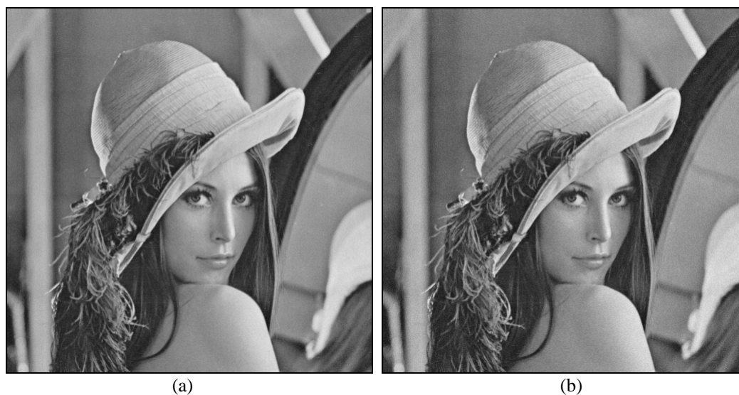
Figure 5. Directly decrypted Lena of reversible scheme (a) \delta = 4 , a total of 4.6 \times 10^4 bits embedded and PSNR = 40.3 dB, (b) \delta = 7 , a total of 7.7 \times 10^4 bits embedded and PSNR = 36.3 dB
