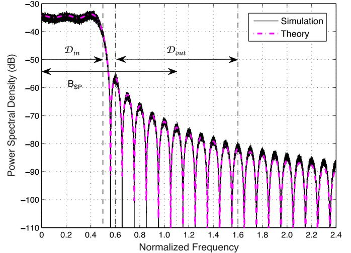
Fig. 5. Averaged PSD of the cancelling pulses with  $n = 5$ ,  $\gamma = 4\text{dB}$ , and  $J = 8$ , where  $\mathcal{D}_{\text{in}}$  and  $\mathcal{D}_{\text{out}}$  are the regions of occupied and adjacent channels, respectively, and  $B_{\text{SP}}$  denotes the channel spacing between them. The bandwidth is normalized by the inverse of the Nyquist interval, i.e.,  $1/T$ , which is equivalent to the bandwidth of the in-band OFDM signal.
