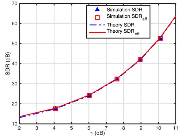
Fig. 7. SDRs with respect to different target PAPR  $\gamma$ .
