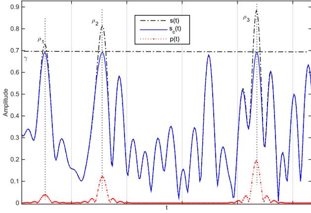
Fig. 2. Example waveforms associated with PC where  $\rho_i$  denotes the envelope level of the  $i$ th peak.
