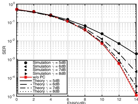
Fig. 11. SER over an AWGN channel with respect to different target PAPR  $\gamma$  of 16-QAM OFDM signals in the presence of PC.
