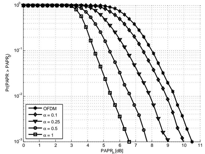
Fig. 7: PAPR performance for 4-QAM when  $\lambda = 0.5$ .
