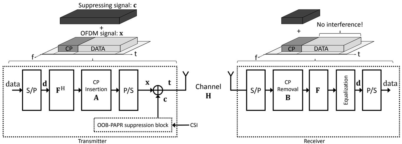
Fig. 1: System model of an OFDM transmitter and receiver with suppressing alignment.
