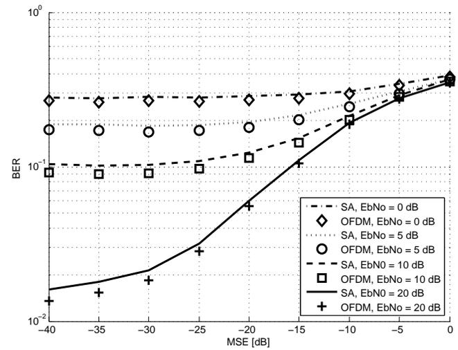
Fig. 11: BER performance for 64-QAM under imperfect CSI,  $\lambda = 0.5$ ,  $\alpha = 0.25$ .
