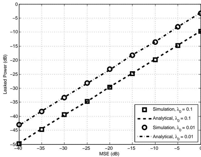
Fig. 9: Leaked power in (29) under imperfect CSI,  $\lambda = 0$ .
