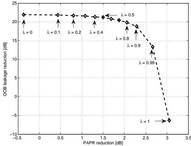
Fig. 3: Performance trade-off between OOB reduction and PAPR reduction when  $\alpha = 0.25$ .
