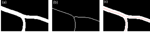
Fig. 2. Vessel centreline refinement process. (a) Vessels from the binary mask. (b) Thinned centrelines. (c) Refined centrelines plotted on the binary vessel mask.
