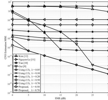
Fig. 3. Performance comparison of different CFO estimators versus SNR when  $f_d = 2.330$ .
