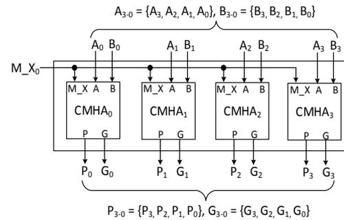
Fig. 3. Structure of a group with four CMHAs.
