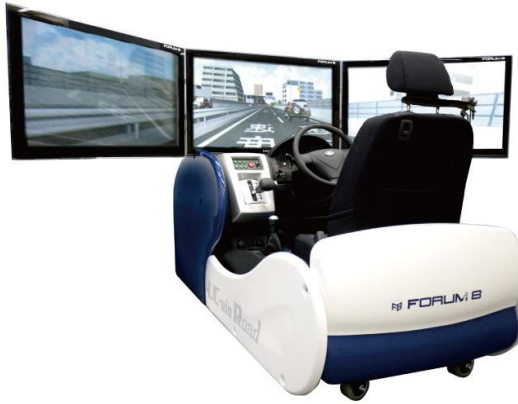
Fig. 2. Primary setup of driving simulator (FORUM8).
