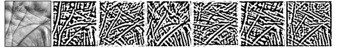
Fig. 5. The learned discriminant direction feature maps. The first image is a palmprint image. The second to seven ones are the learned DDBC maps of the first to six levels, respectively.
