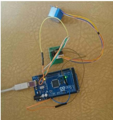
Fig 4. Arduino Mega 2560 + Stepper Motor and its drive.
