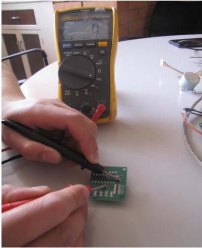
Fig 3. Checking Connections.
