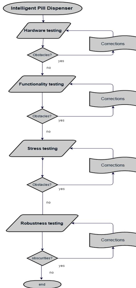
Fig 2. Testing Intelligent PillBox Flow Diagram
