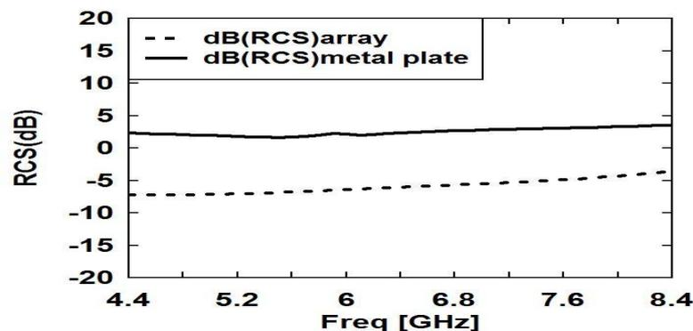
Fig. 6: A comparison between the bistatic RCS of a PEC tile and an absorbing tile designed at resonance frequency 6.3 GHz.
