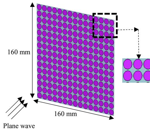
Fig. 4: Finite tile of absorber.
