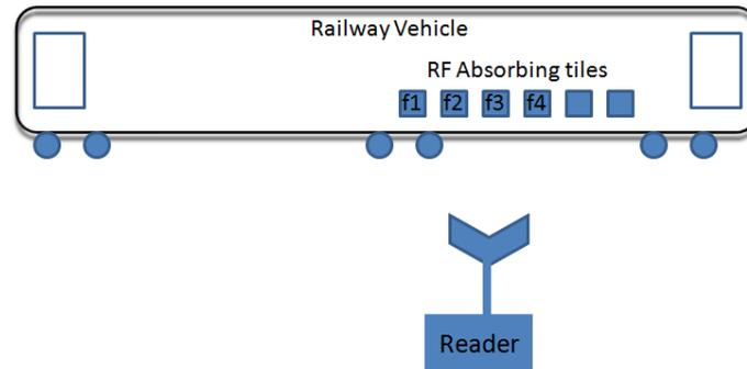
Fig. 1: Schematic diagram of the proposed passive RFID system for railway vehicles based on Narrow band absorbing tiles
