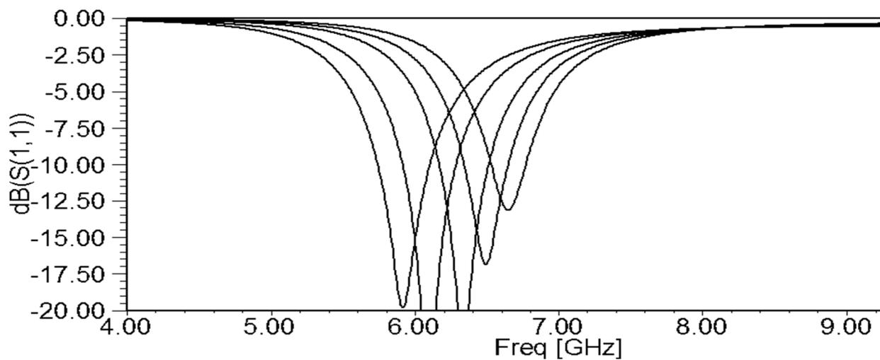
Fig. 3: Reflection coefficients for samples of designed infinite array absorbers
