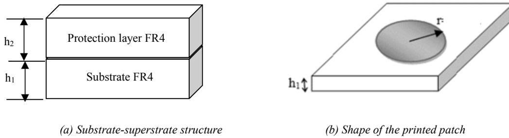
Fig. 2: Geometry of the unit cell
