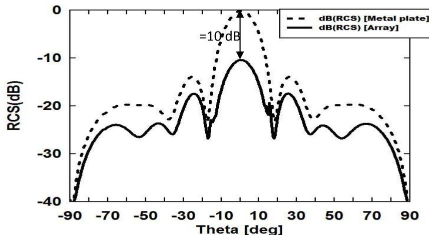
Fig. 5: A comparison between the bistatic RCS of a PEC tile and an absorbing tile designed at resonance frequency 6 GHz
