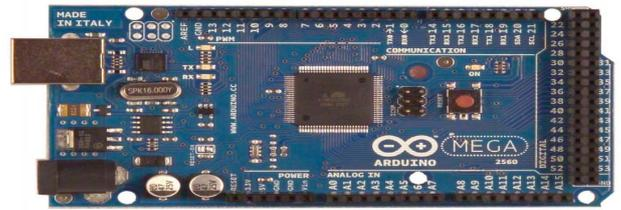
Fig.6. Arduino Mega 2560 [6]
