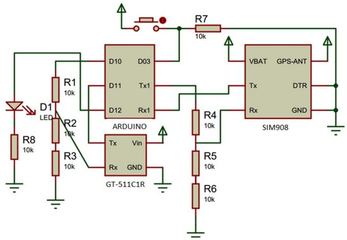
Fig. 5 Schematic diagram of in-vehicle tracking unit.
