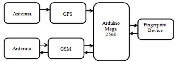
Fig.4 Block diagram of vehicle tracking system with fingerprint verification.
