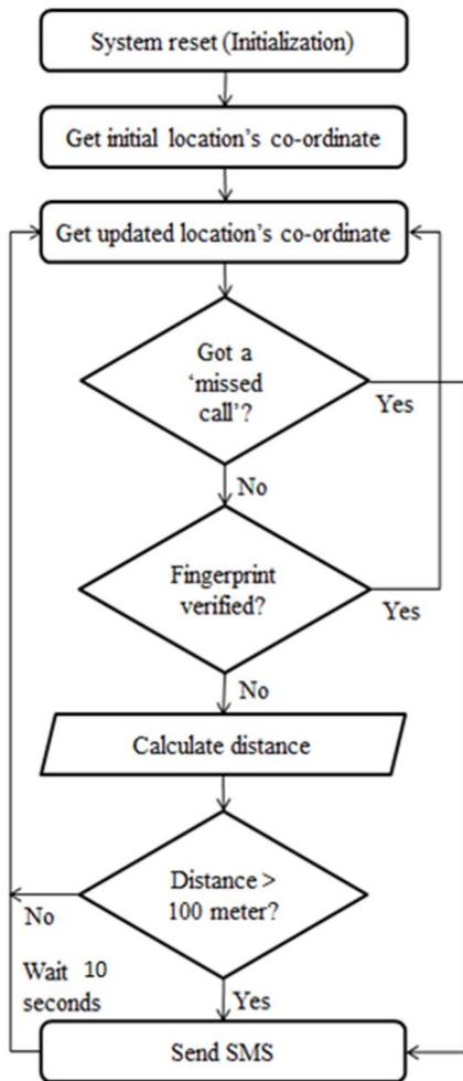
Fig. 3 Flow chart of security check and sending SMS.
