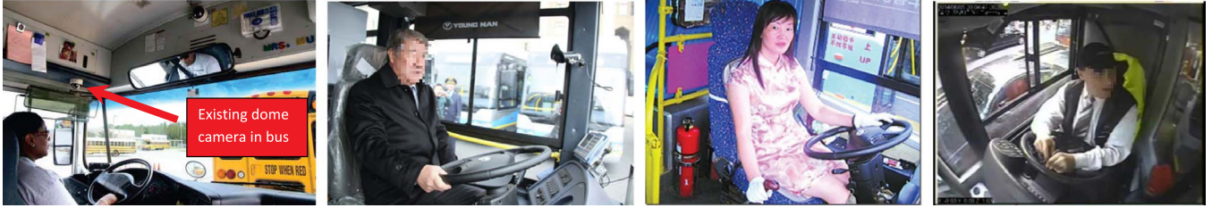
Fig. 1. Existing dome camera in the bus and example images of bus drivers captured by the dome cameras in buses. Only an oblique view of low-resolution face images can be captured by the existing dome cameras for normal driving poses. (Images came from open sources of bus service companies with face portions of the drivers being pixelated for keeping anonymity.).
