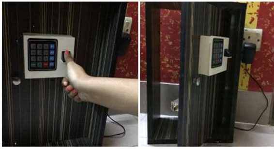
Fig. 6. Fingerprint sensor based door lock.
