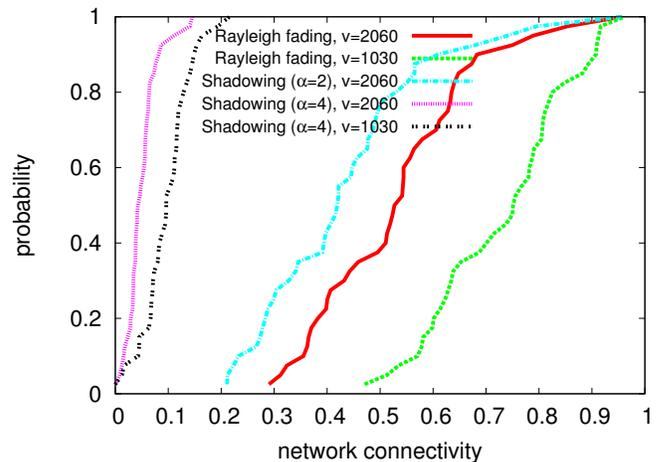
Fig. 3. Simulation results of network connectivity for different propagation models and vehicular subscriber densities.
