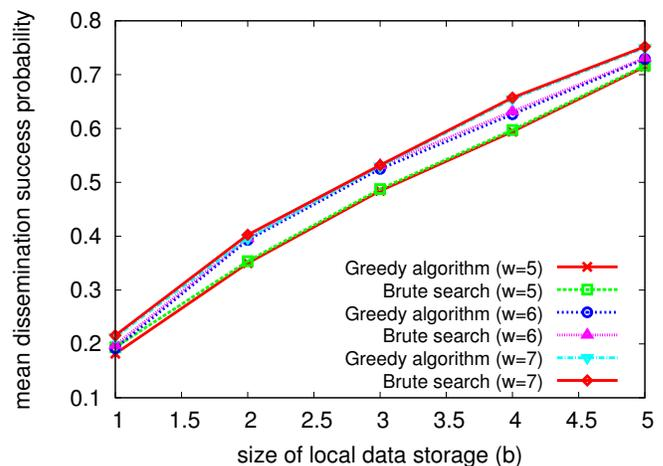
Fig. 9. Mean dissemination success probability of all vehicle-data chunk pairs with respect to the data storage size for the proposed greedy and the brute search algorithms (Rayleigh fading,  $v = 2060$ ,  $u = 6$ ).
