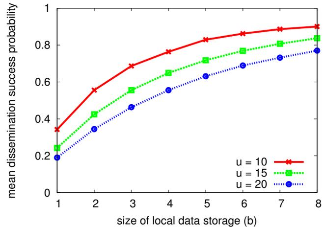
Fig. 6. Mean dissemination success probability of all vehicle-data chunk pairs with respect to the size of local data storage (Rayleigh fading,  $v = 2060$ ).
