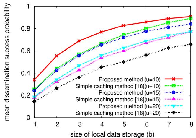
Fig. 7. Mean dissemination success probability of all vehicle-data chunk pairs with respect to the storage size for the proposed and the simple caching methods (Rayleigh fading,  $v = 2060$ ).
