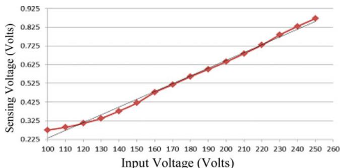
Fig. 4. Scaling factor ( $m_1$ ) of voltage signal.
