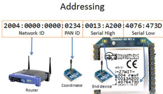
Fig. 8. Address transformation from ZigBee sensing unit to Internet packet.
