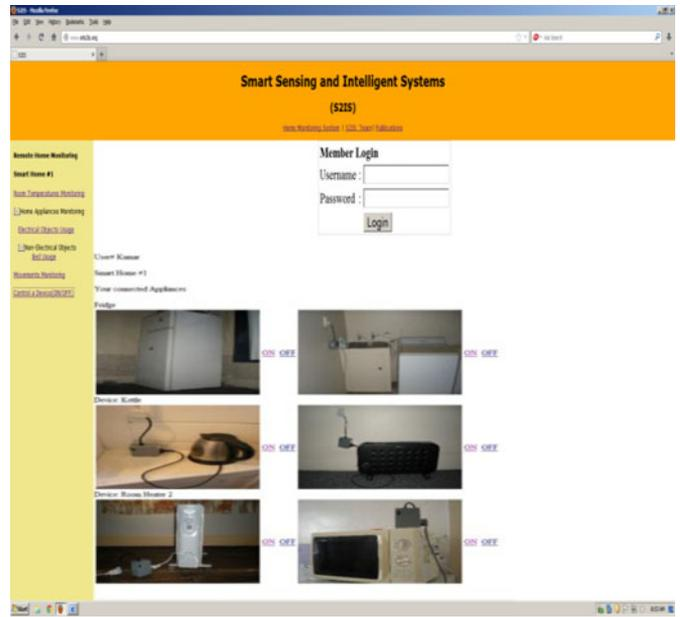
Fig. 12. Secured webpage for controlling appliances remotely after successful authorized login.
