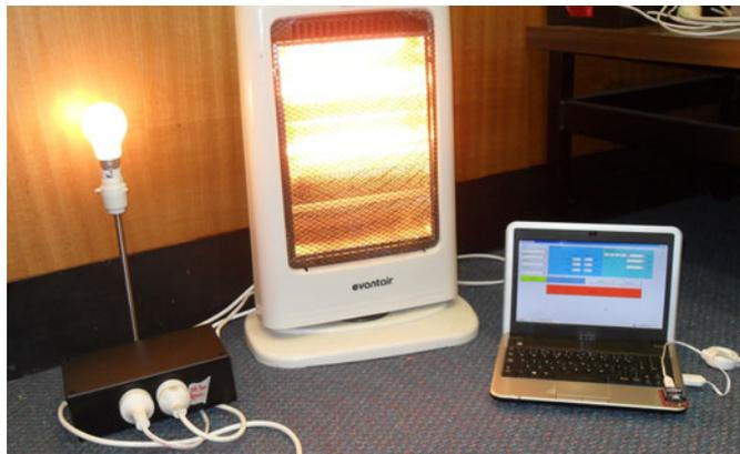
Fig. 9. Smart power monitoring and control system at the residence.
