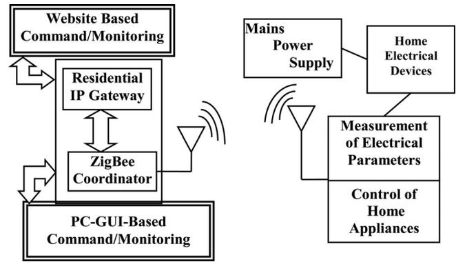
Fig. 1. Functional block diagram of the system.
