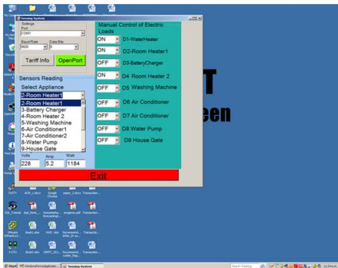
Fig. 10. Graphical user interface of smart power monitoring and control system at the local residence.
