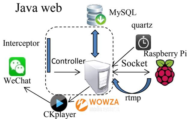
Fig.2. Software Architecture
