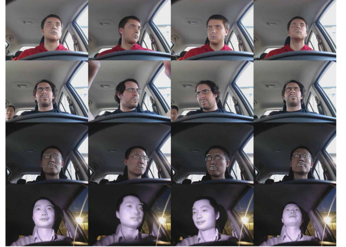
Fig. 5. SDM landmark detection under different poses, illuminations, and ethnicities.
