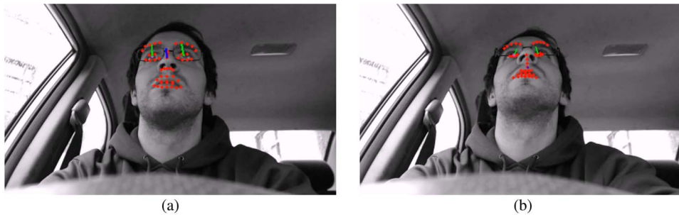
Fig. 14. Illustration of tracking failure due to extreme pose and glasses. Green lines starting at driver’s eyes show the estimated gaze direction. The blue line starting at the driver’s nose shows the estimated head pose orientation. a) Driver looking at the windshield top left. b) Driver looking at the driver visor position.
