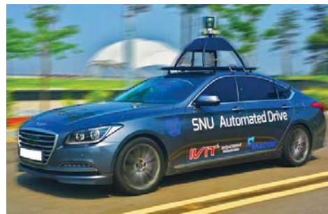
Fig. 6. Probe vehicle equipped with a 3D Lidar and a GPS+INS positioning system.
