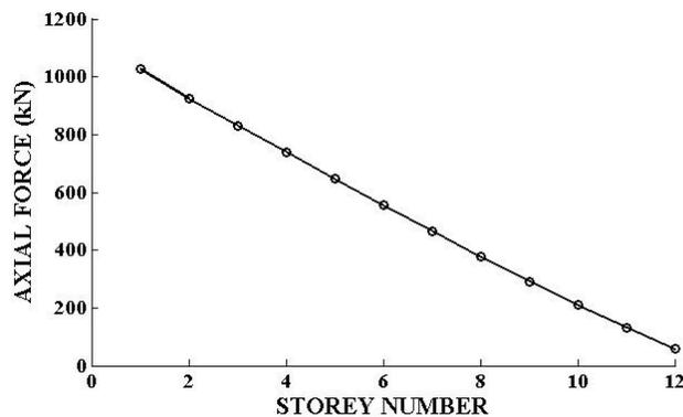
**Figure 5:** Axial force on shear wall
