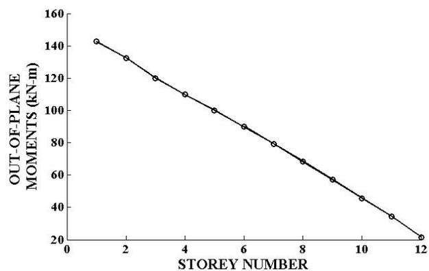
**Figure 6:** Out of plane moments on shear walls
