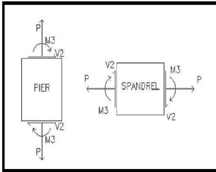
**Figure 4:** Pier and Spandrel forces in ETABS
