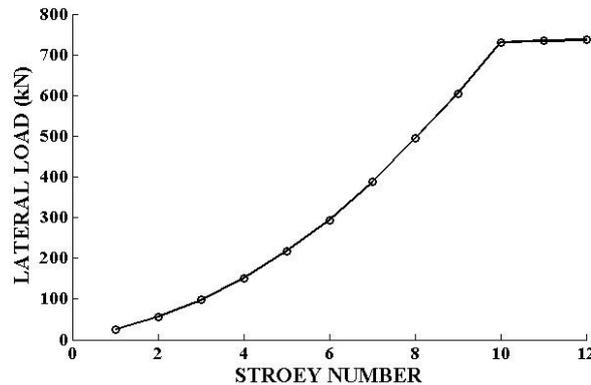
**Figure7:** Lateral loads on shear walls
