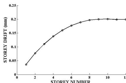
**Figure 9:** Storey drifts on shear walls
