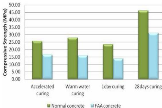
Compressive strength of normal and FAA concrete
