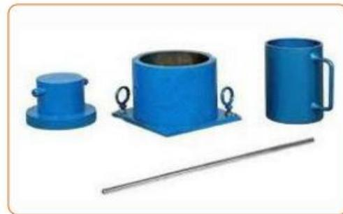
Aggregate crushing value apparatus
