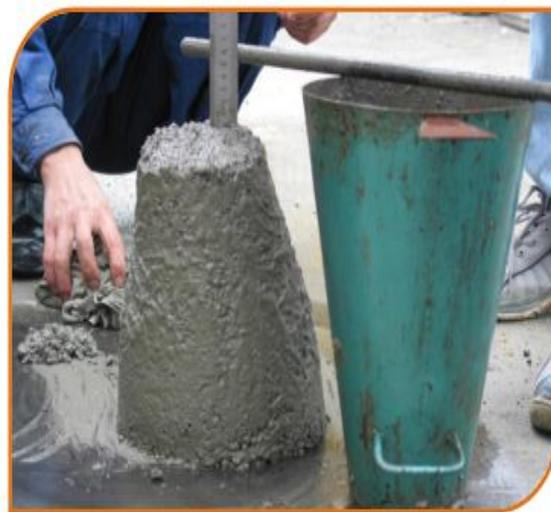
Slump cone test
