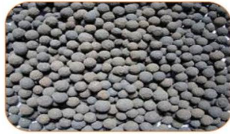
Sintered Fly ash aggregates
