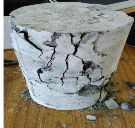
Failures of cylinders
