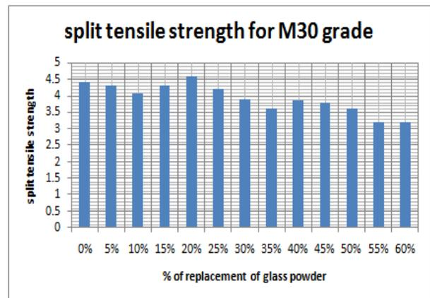
**SPLIT TENSILE STRENGTH OF CONCRETE**
