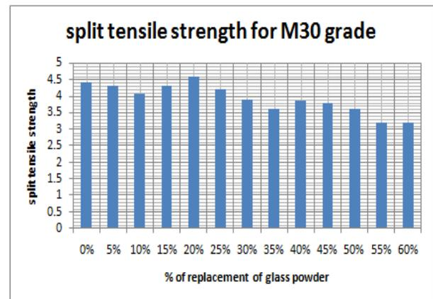
**SPLIT TENSILE STRENGTH OF CONCRETE**
