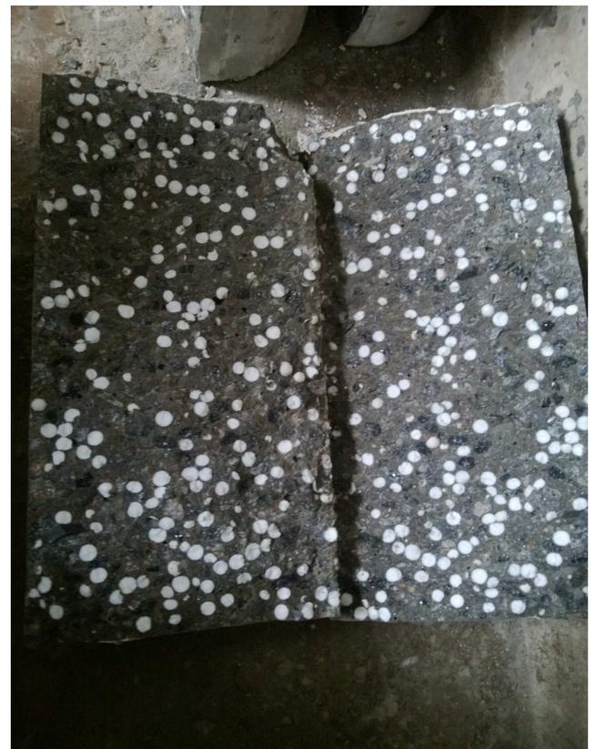
**Fig. 2: Broken surfaces of failed cylinders**
