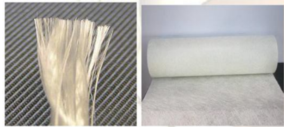
Glass Fiber in Strand Form Glass Fiber in Mat Form EXPERIMENTAL PROGRAM AND MIX DESIGN
