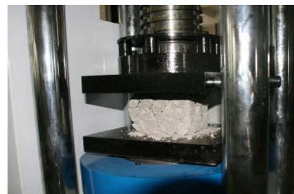
Compressive strength of geopolymer concrete equipment
