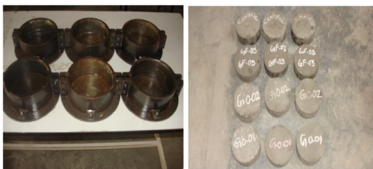
Moulds used for casting specimens for impact test
