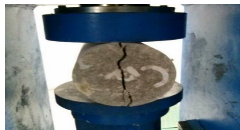
Split tensile strength of geopolymer concrete equipment
