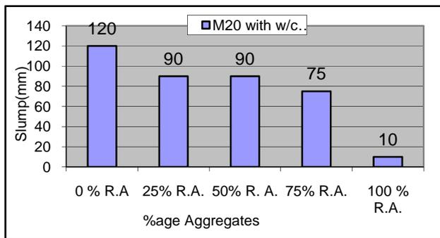
Fig. 5 Slump value of M20 concrete with w/c=0.650
