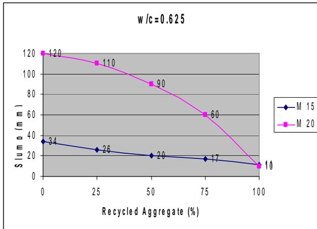
Fig. 4 Slump value of M15 & M20 concrete with w/c=0.625
