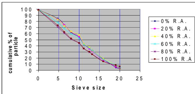
Fig. 1 Average sieve analysis test of aggregates
