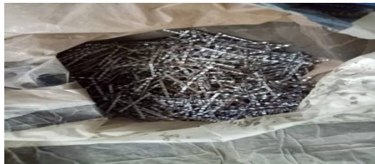
Figure 2:Crimped Steel Fibre
