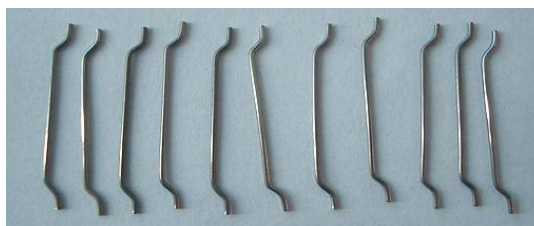
Figure 3:Hooked Steel Fiber
