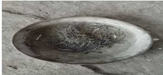
Figure 1: Straight Steel Fibres
