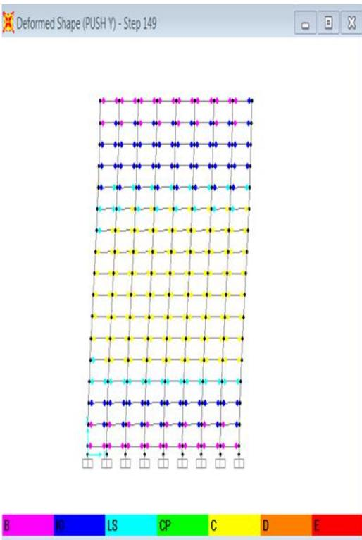
**Fig.14** Hinge formation at performance point in Y direction for regular shape building (G+15)
