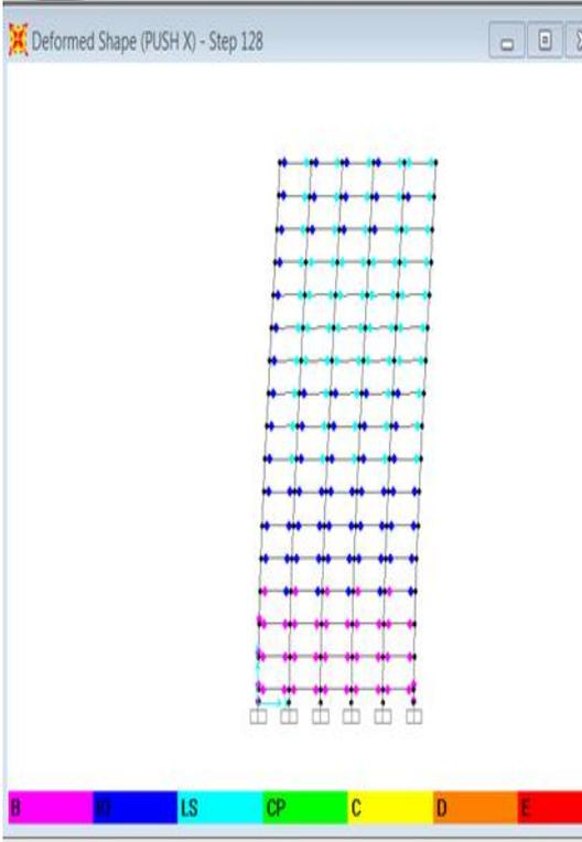
**Fig.13** Hinge formation at performance point in X direction for regular shape building (G+15)
