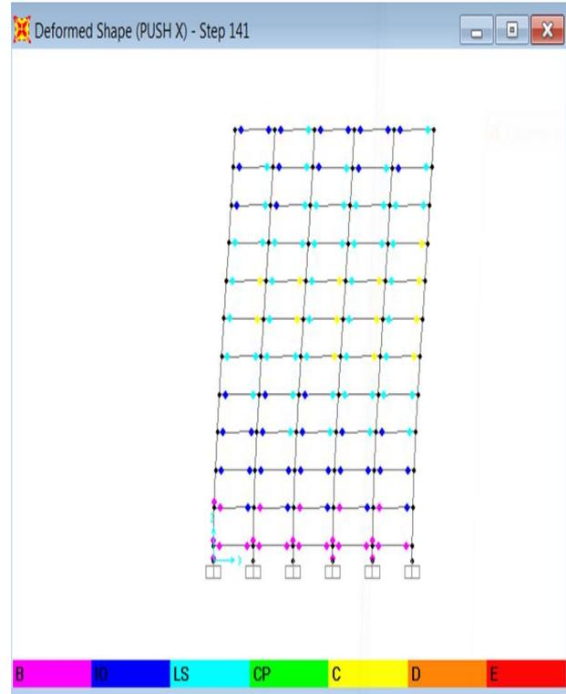
Fig.11 Hinge formation at performance point in X direction for 40/25 building (G+10)
