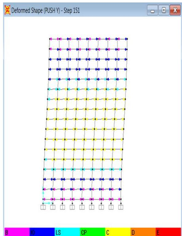
**Fig.16** Hinge formation at performance point in Y direction for 40/25 building (G+15)
