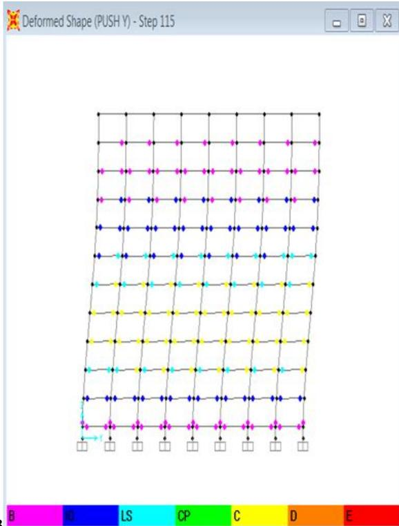
Fig.10 Hinge formation at performance point in Y direction for regular shape building (G+10)
