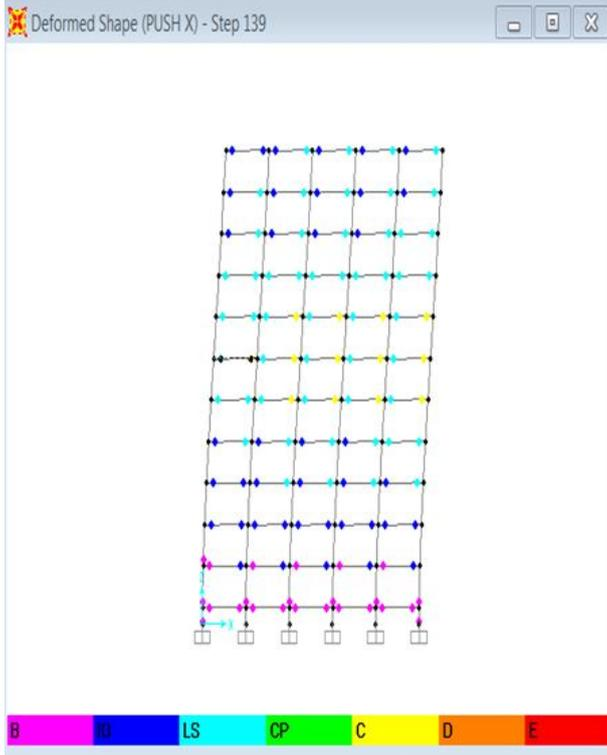
Fig.9 Hinge formation at performance point in X direction for regular shape building (G+10)
