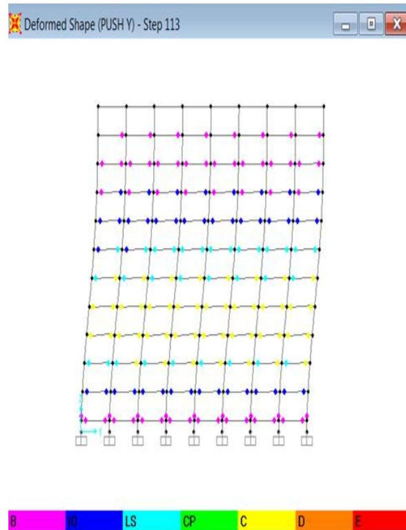
Fig.12 Hinge formation at performance point in Y direction for 40/25 building (G+10)
