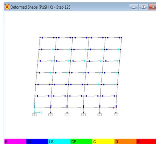
**Fig.7 Hinge formation at performance point in X direction for 40/25 building (G+5)**
