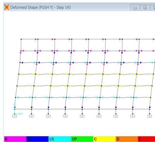
**Fig.8 Hinge formation at performance point in Y direction for 40/25 building (G+5)**
