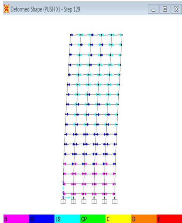
**Fig.15** Hinge formation at performance point in X direction for 40/25 building (G+15)
