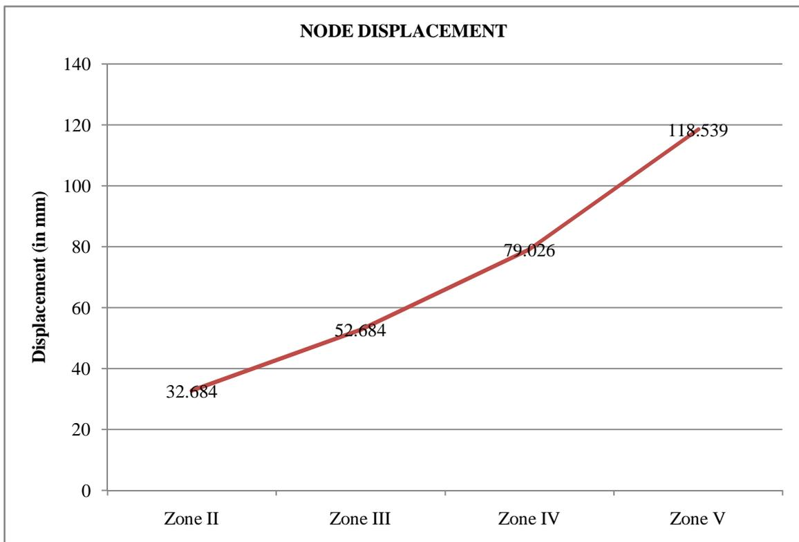
Figure 6:- Maximum Node Displacements
