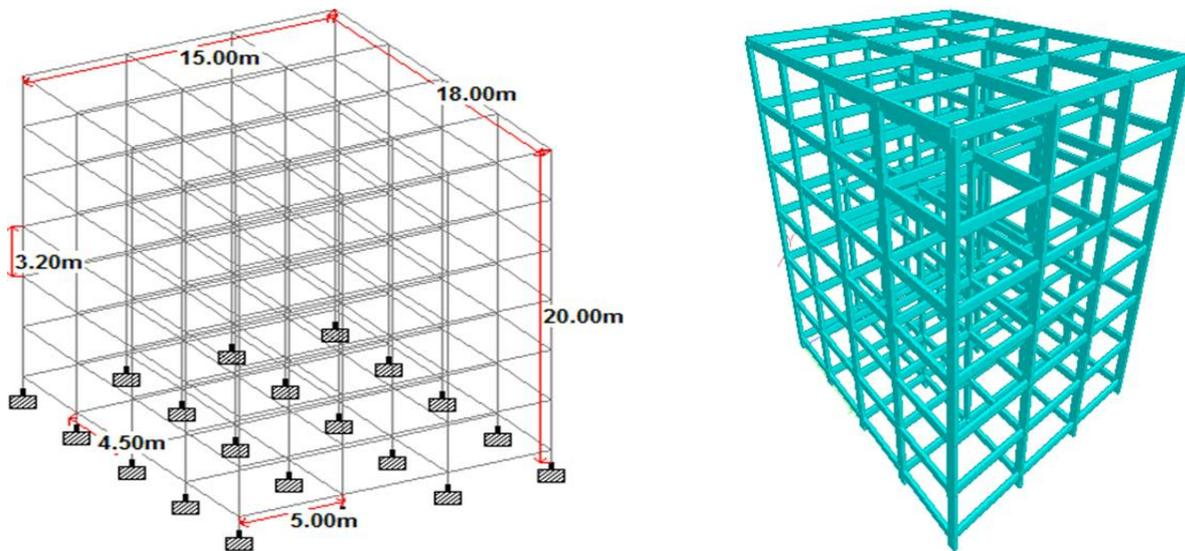
Figure 1:- Typical 3D view and Rendering View of Building
