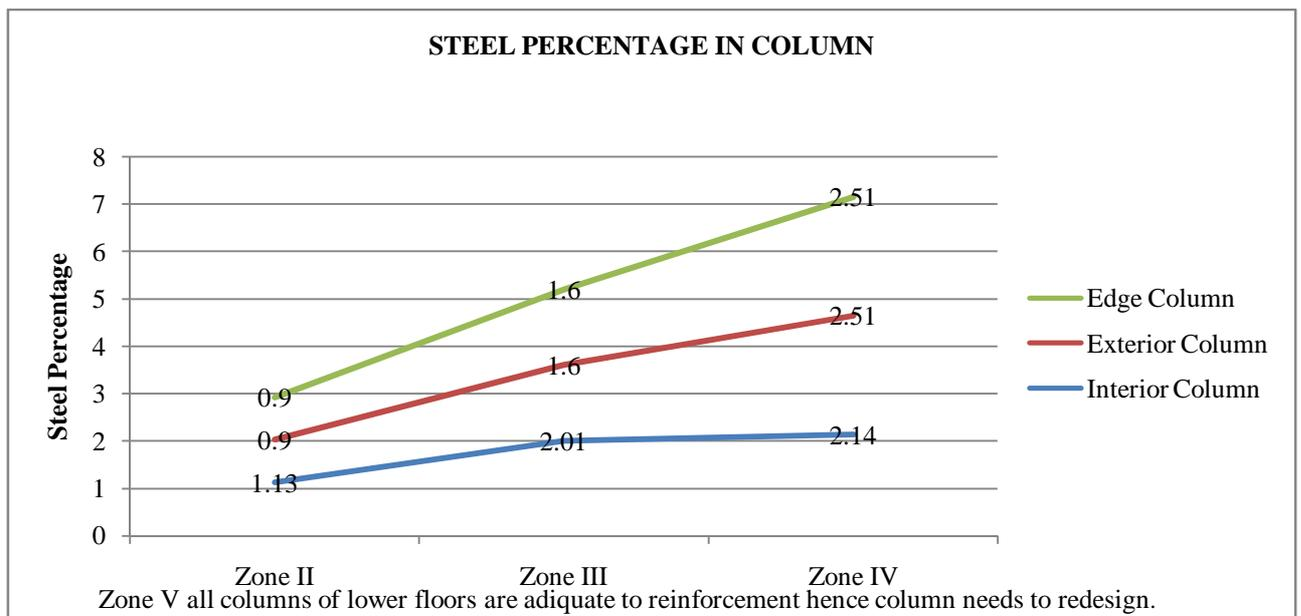
Figure 2:- Maximum Percentage of Steel in Columns
