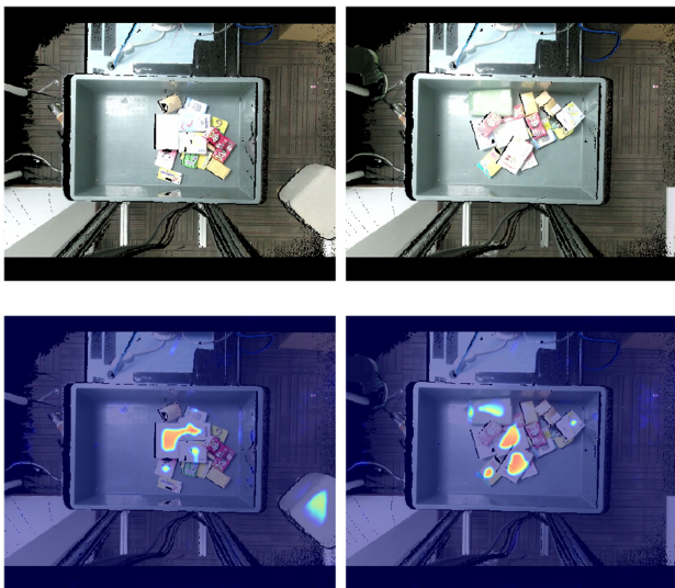
Fig. 1. Some failure affordance cases: The top panel shows the original images captured by the global camera and the bottom panel shows the affordance maps. In the case of clutter (left) or occlusion (right), using the conventional affordance calculation may result in mistake proposals.
