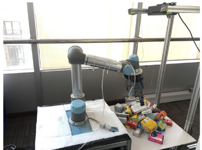
Fig. 9. Physical experimental platform, which contains a Kinect camera as a vision sensor, a UR5 manipulator with the developed composite robotic hand.
