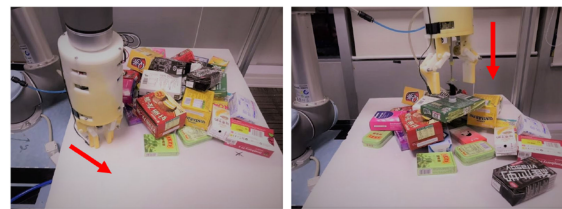
Fig. 18. Some failure cases of the proposed interactive perception method. Left: DQN produces useless pushing action (the dashed arrow), which does not change the operation scene. Right: Object to be picked lacks sufficient support.
