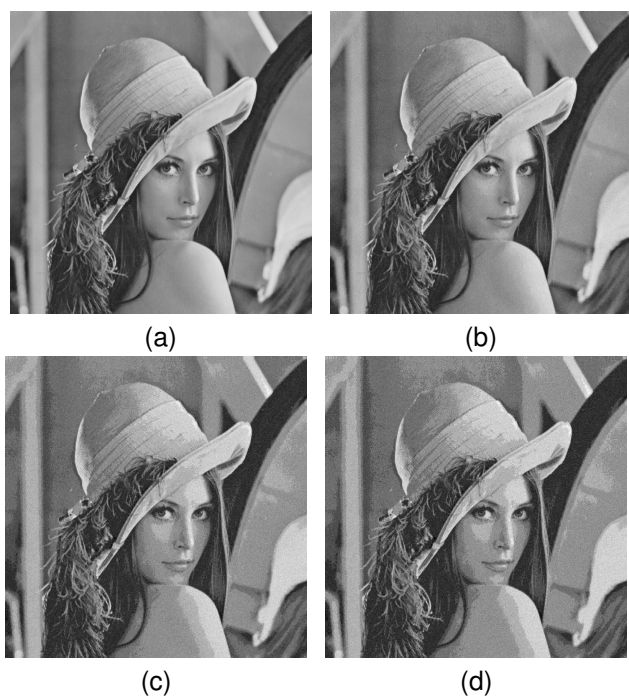
Fig. 11. The distortion of image under bit-flipping attack. The peak signal to noise ratio (PSNR) and structural similarity image measurement (SSIM) of the watermarked and attacked images are calculated to quantifiably show the image quality. (a) original image, (b) watermarked image, PSNR = 34.2603dB , SSIM=0.8531 , (c) watermarked image after bit-flipping attack with 30% bits flipped, PSNR = 27.6602dB , SSIM=0.6085 , and (d) watermarked image after bit-flipping attack with 40% bits flipped, PSNR = 26.6603dB , SSIM=0.5670 .
