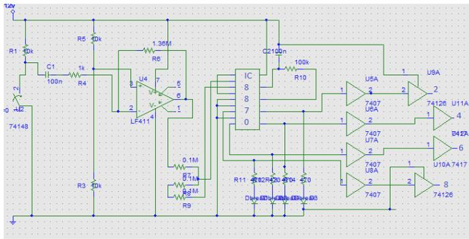
Figure 2. Circuit diagram of the DTMF operation
