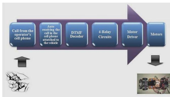
Figure 1. Block diagram of GSM network controlled vehicle.
