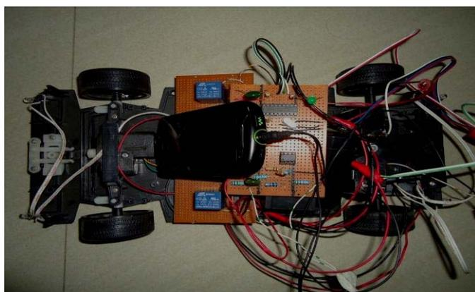
Figure 6. Implemented GSM controlled vehicle
