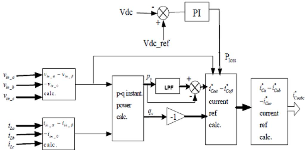
Figure 3: Control block diagram of shunt APF
