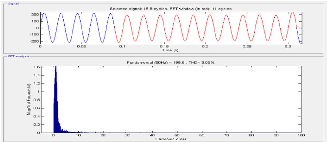
Figure 8: Total harmonic distortion analysis of source voltage
