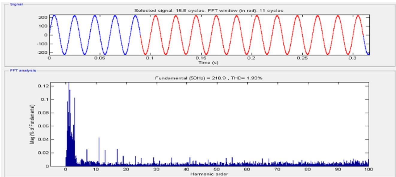
Figure 9: Total harmonic distortion analysis of line voltage
