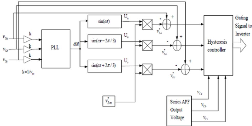
Figure 2: Control block diagram of series APF
