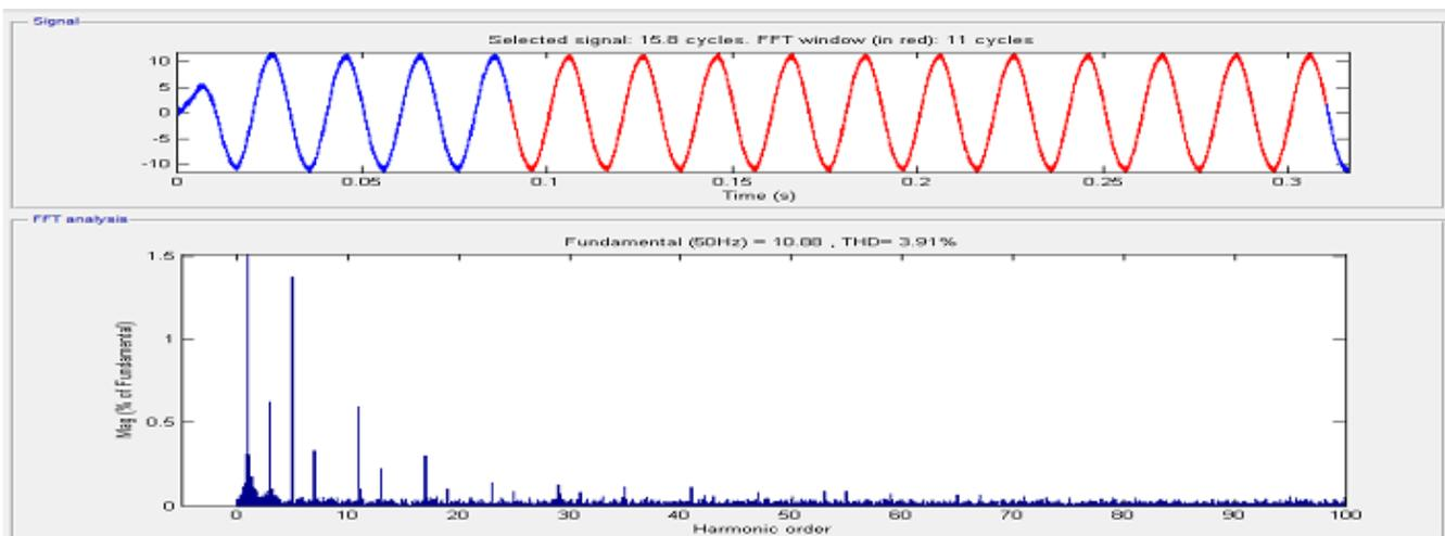
Figure 11: Total harmonic distortion of line current.
