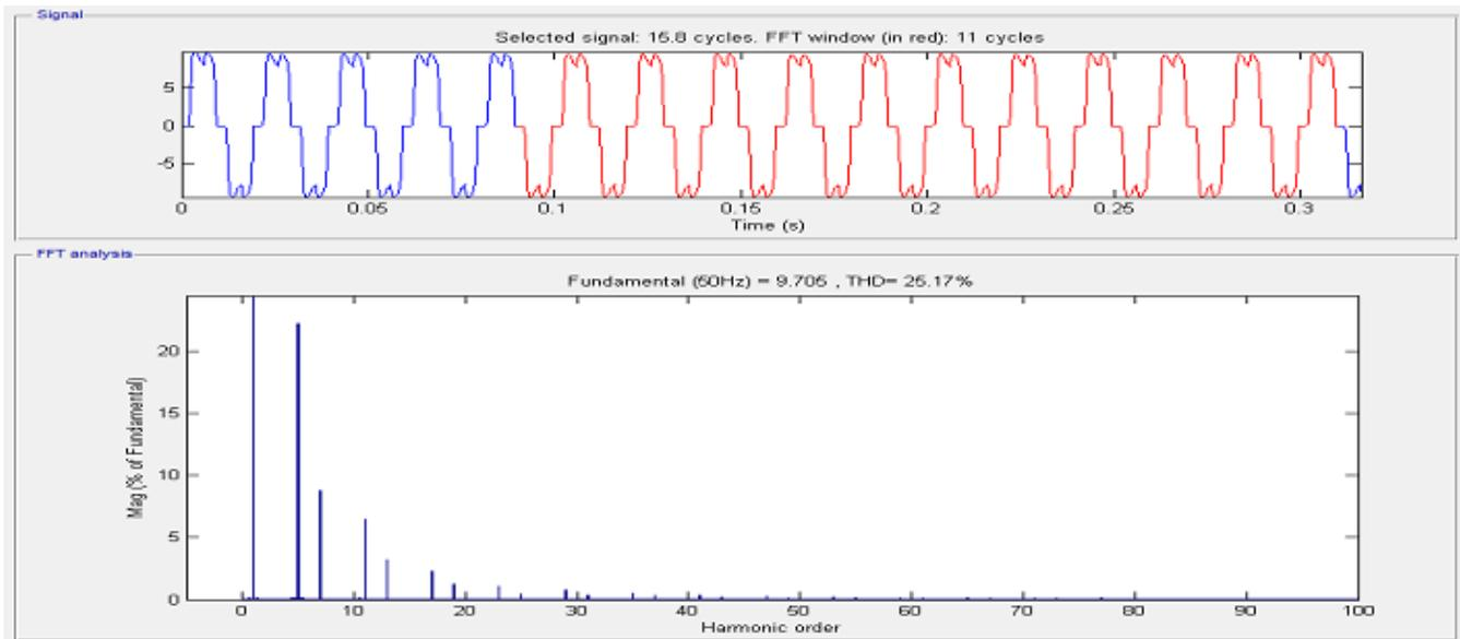
Figure 10: Total harmonic distortion of load current
