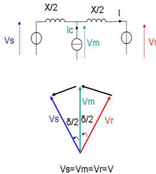
Fig. 3: Shunt compensation
