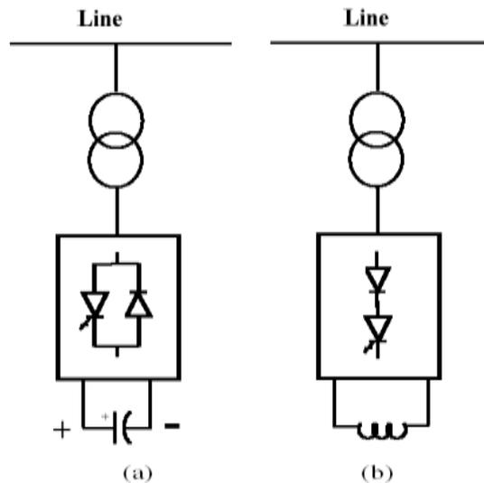
**Fig 1: Static Synchronous Compensator (STATCOM) based on
