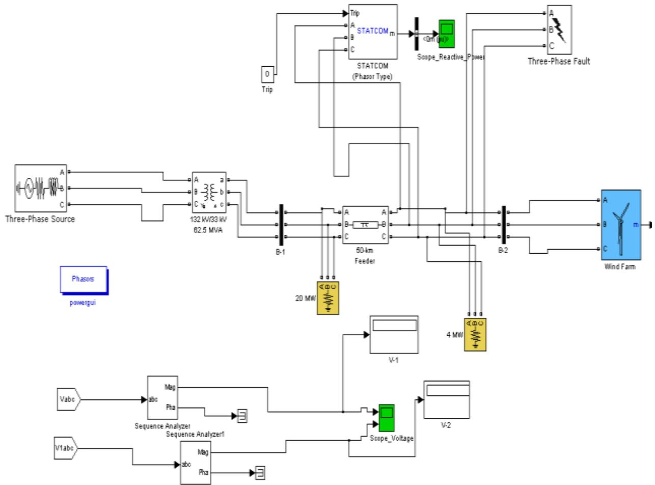
Fig. 5: Simulink Model of IG with STATCOM
