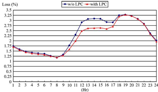
Fig. 15. Percentage of system power loss before and after applying LPC for loading balance (with PV system).
