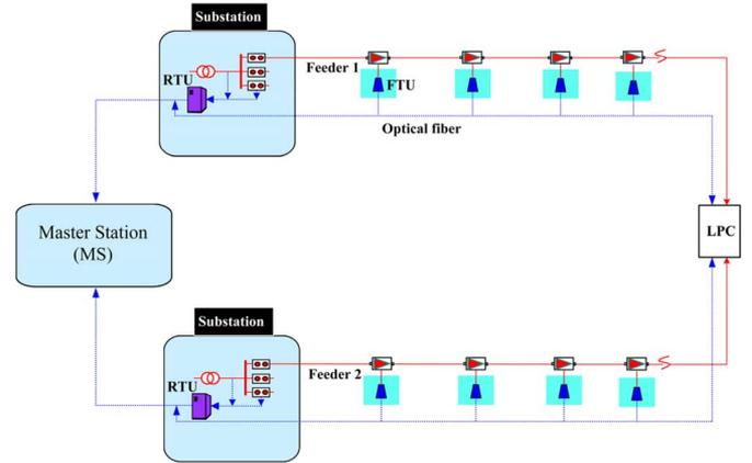
Fig. 1. Distribution automation system with a loop power controller.
