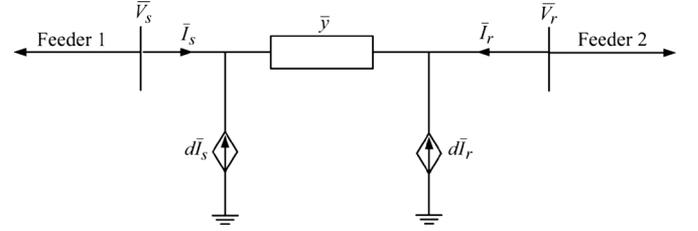
Fig. 4. Modified equivalent circuit model of LPC.
