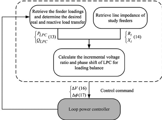
Fig. 2. Flowchart of LPC control algorithm.
