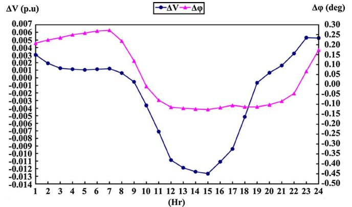
Fig. 12. Voltage ratio and phase shift for the power transfer by LPC (without the PV system).
