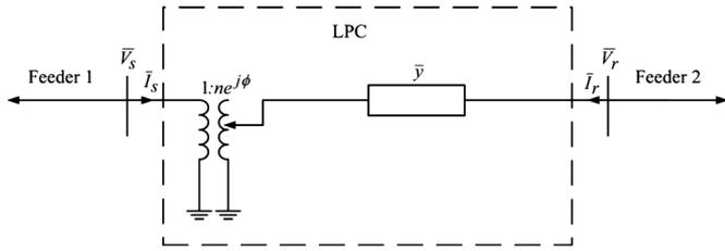
Fig. 3. Circuit model of loop power controller.
