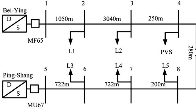
Fig. 6. Taipower distribution feeders for computer simulation.
