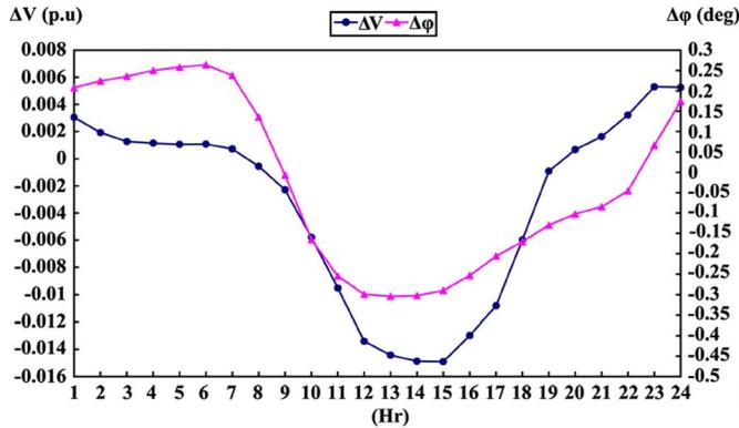
Fig. 13. Voltage ratio and phase shift with the control of LPC (with PV system).
