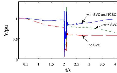
(a) The generator terminal voltage
