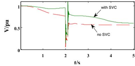
Figure 6. Terminal voltage with and without SVC compensate
