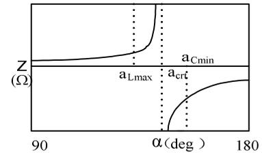
Figure 4. Operating characteristic curve of TCSC
