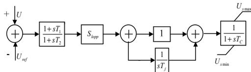
Figure 2. Controller diagram of SVC
